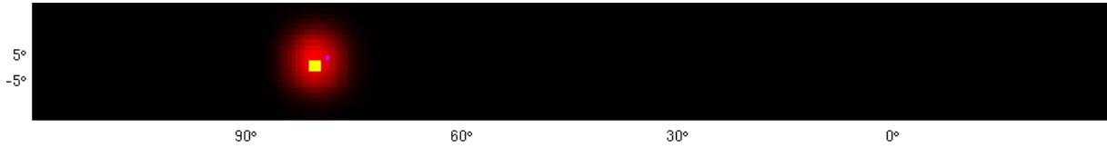
Figure 4: Backprojection of the captured images onto the surface of a parametrized cylinder. The captured specular highlight (red) matches the predicted reflection point ( \theta_o = \theta_i , yellow).
